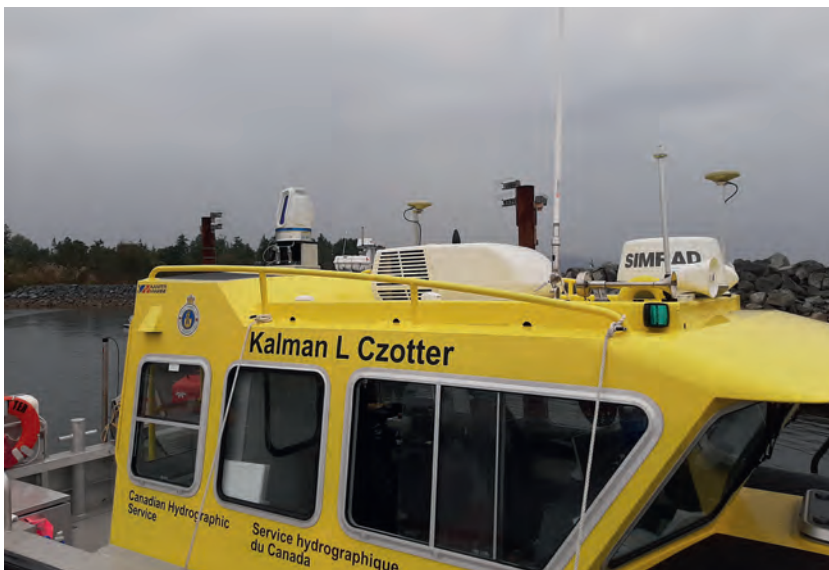
▲ Example installation of the Optech Polaris laser scanner on a coastal survey vessel. Image courtesy of the Canadian Hydrographic Service.
